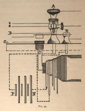
the coil, the current, as it passes over the wire of this primary coil, renders magnetic both the centre bundle of soft iron wires and the soft iron rod.
